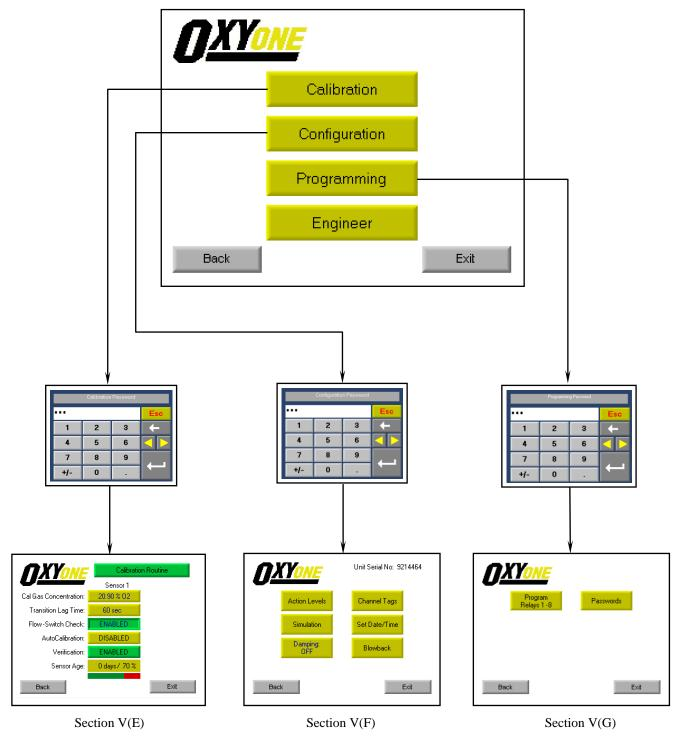
By touching the Calibration, Configuration or Programming buttons on the Menu screen shown above, access is gained to that sub-menu. The Engineer sub-menu is reserved for Ntron use only.
