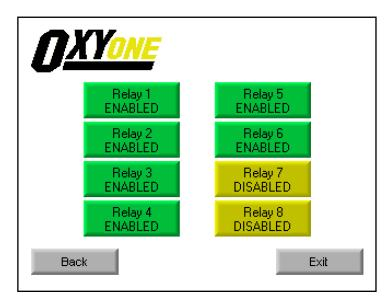
Touch any of the Level buttons (1-8) to enter into a sub-menu for that Relay. The following screen will load. (Relay 1 shown as an example below).
